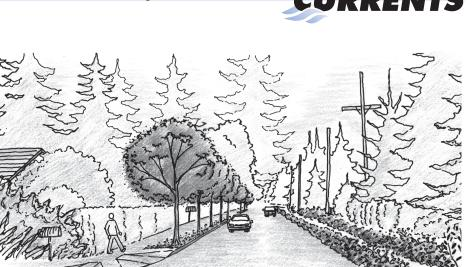
Typical road improvements on 3rd Ave. NW north of NW 180th St. include a six-foot sidewalk and four-foot planter strip (where feasible) along the west side of 3rd Ave. NW with landscaping and gravel parking strip along the east side.
