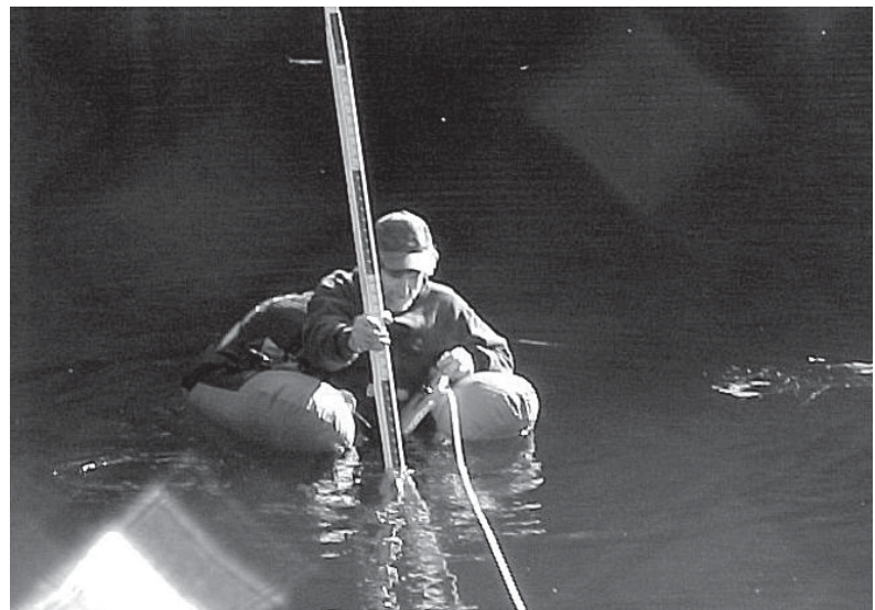
Shoreline Water Quality Specialist Andy Loch uses a floating fisherman inner tube to measure the lake bottom at Hidden Lake following a recent dredging. Located in Shoreview Park, Hidden Lake's forebay accumulates an average of 180 cubic yards of sediment each year. The sources of sediment are Boeing Creek, channel erosion and impervious roads. Shoreline dredges the lake every one to two years to protect downstream water quality. After dredging, City staff measure the lake contours to determine how the dredging has affected the lake bed.
