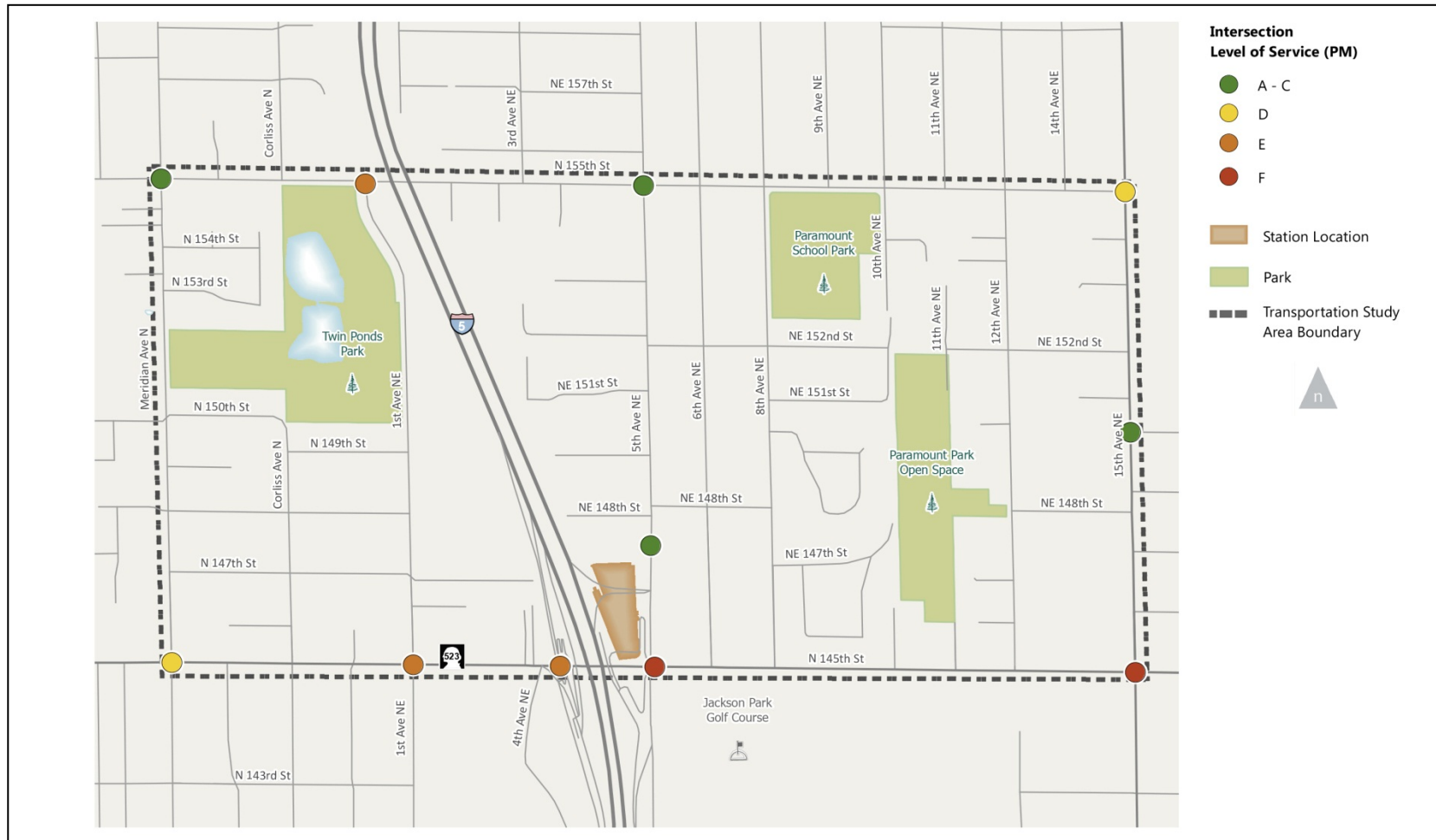
Figure 3.3-9 Intersection Level of Service (Alternative 1—No Action)
