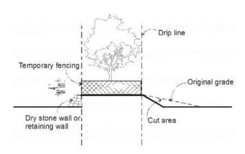
Figure 20.50.370: Illustration of standard techniques used to protect trees during construction.
