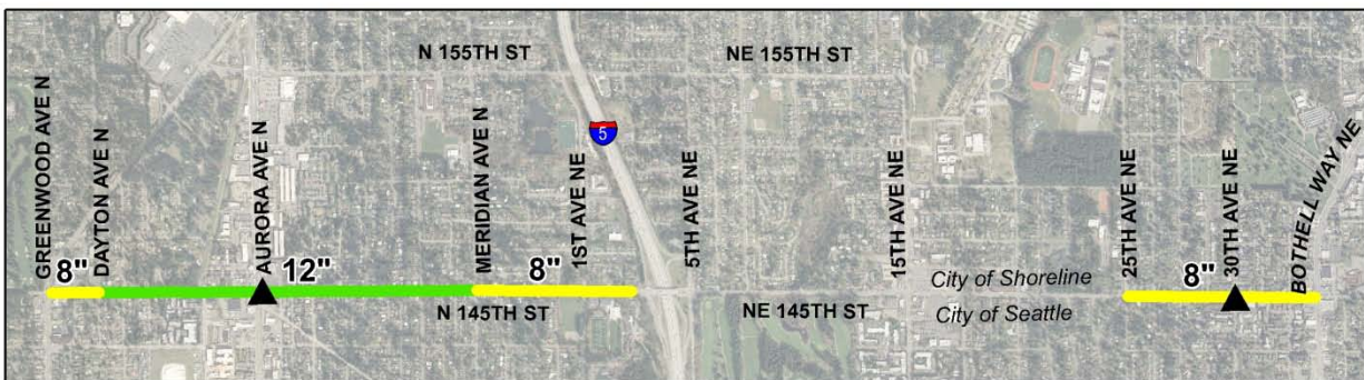
Figure 18- New mains and connections, Alternative B3
