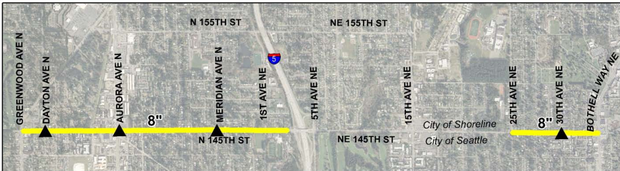
Figure 19- New mains and connections, Alternative B4
