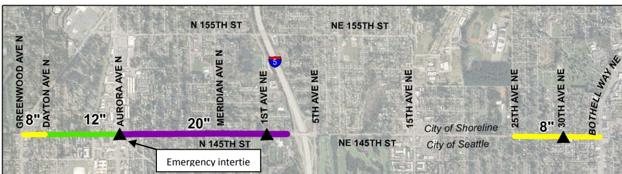
Figure 17- New mains and connections, Alternative B2
