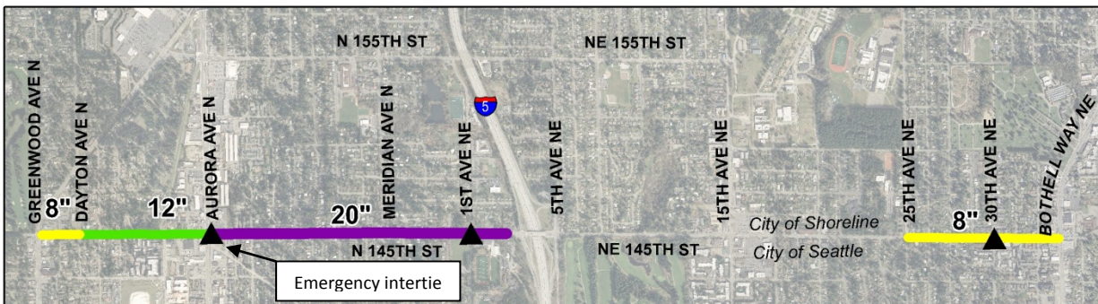
Figure 17 - New Mains and Connections, Alternative B2
