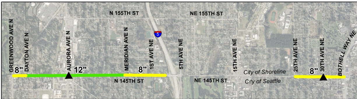
Figure 18 - New Mains and Connections, Alternative B3
