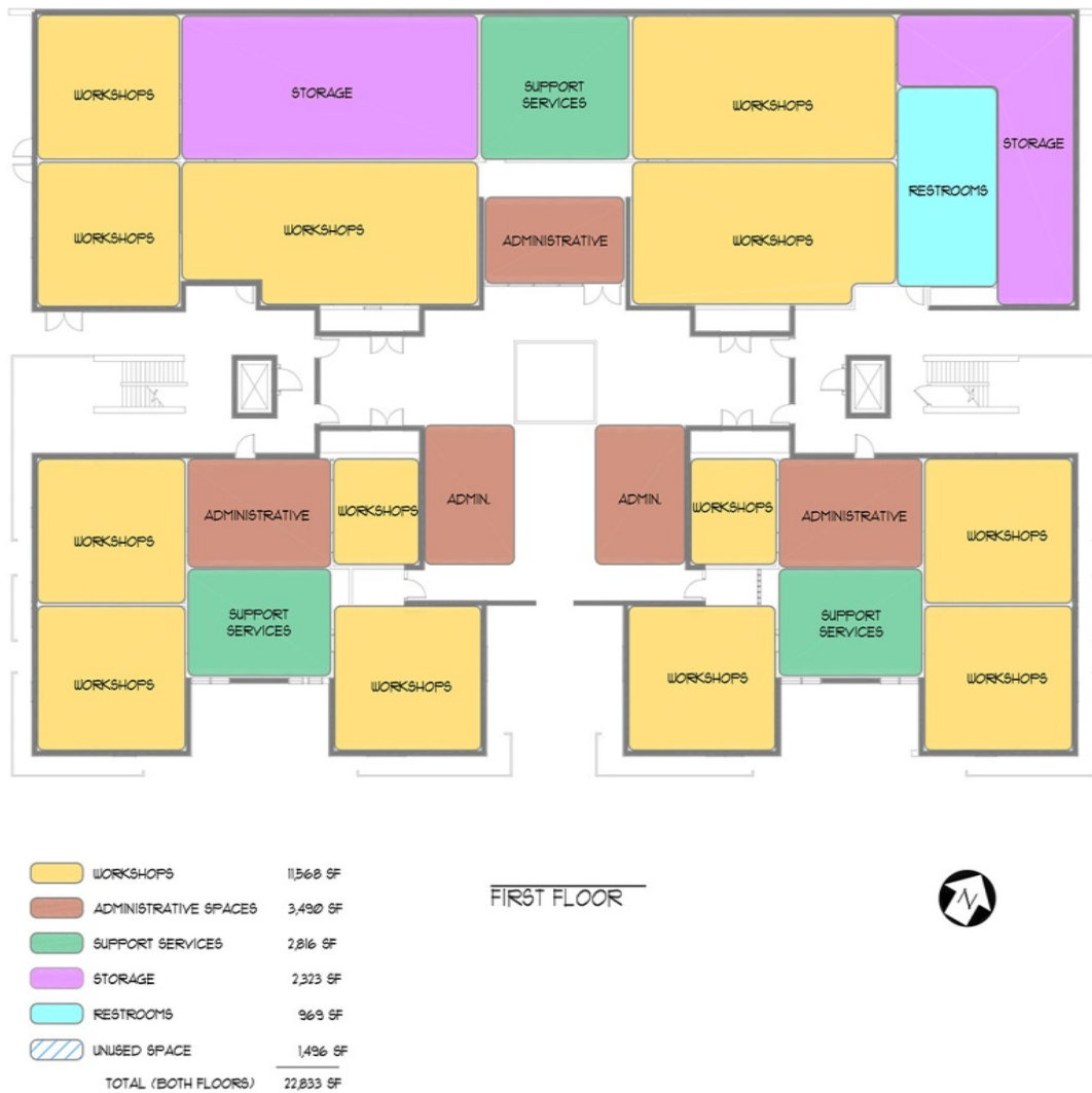
Figure 21: ATP Potential Improvements – ATP Functions - Option 1 – Potential Expansion of Building #66 General First Floor Layout
