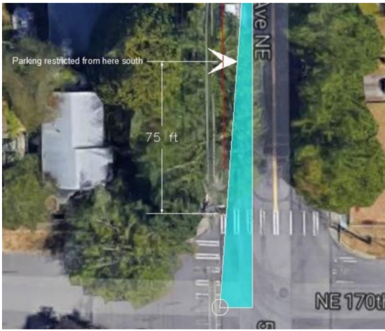
Figure 7. Example sight line diagram at 5th Ave NE/NE 170th St
