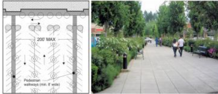
Parking Lot Walkway
