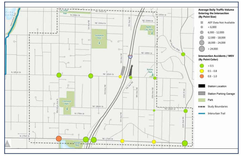
FIGURE 3-8: Accident Rate (Existing Conditions)
