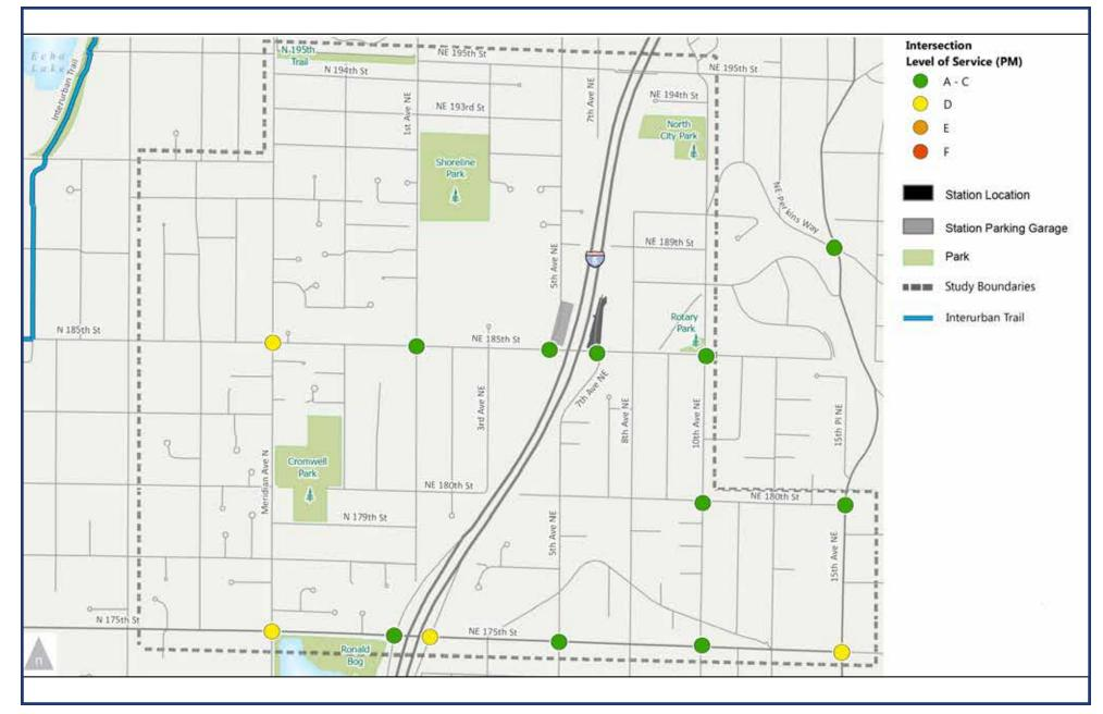
FIGURE 3-7: Intersection Level of Service (Existing Conditions)
