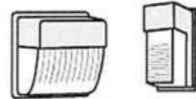
Unshielded Wallpacks & Unshielded or Poorly-shielded Wall Mount Fixtures
