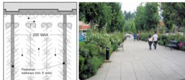
Parking Lot Walkway
