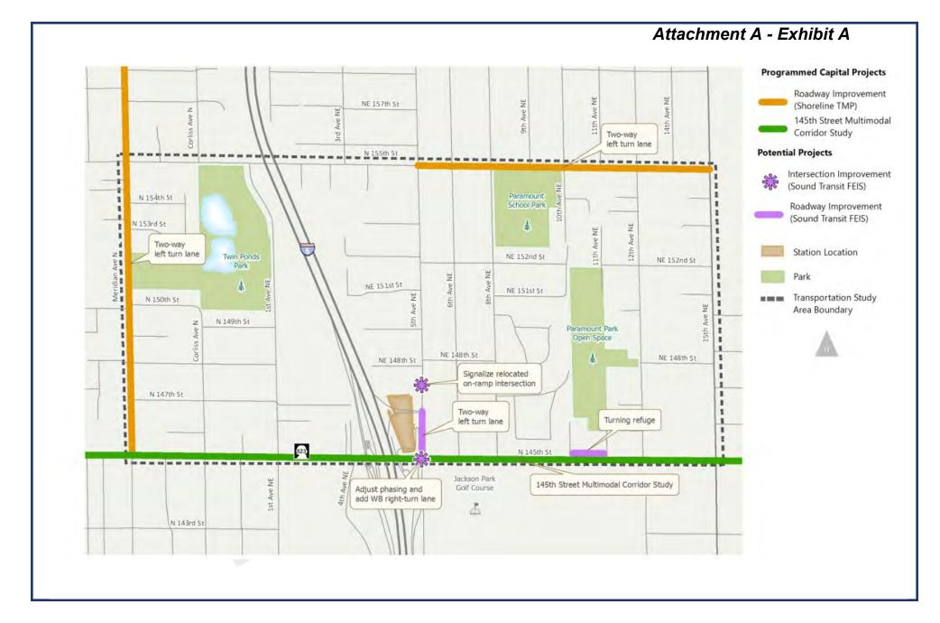
FIGURE 3-14: Roadway Improvements to Accommodate Growth Identified in the Transportation Master Plan
