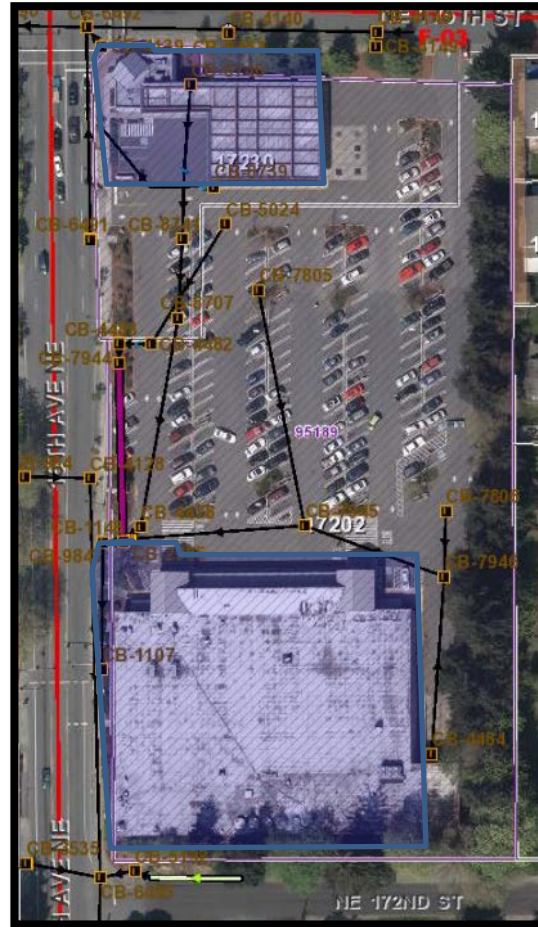
Figure 2 – 3.25 Acre Commercial Property with 1.5 Acre permeable pavement parking lot
