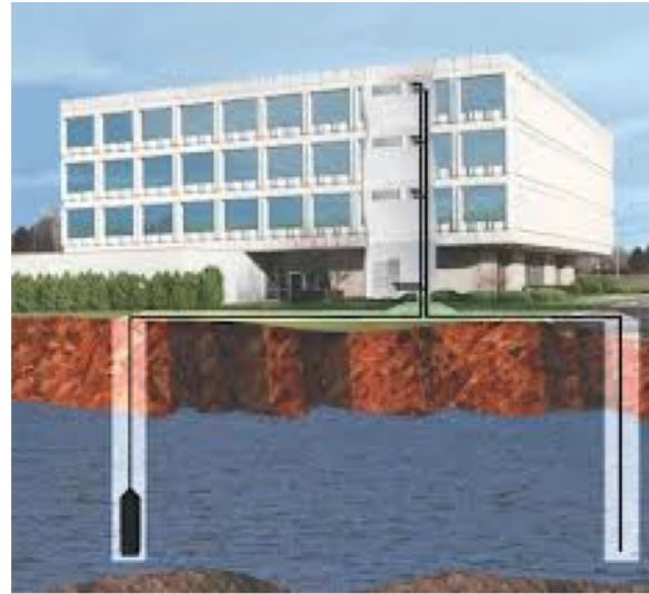
Figure 6 — Ground-Source Heat Pump
