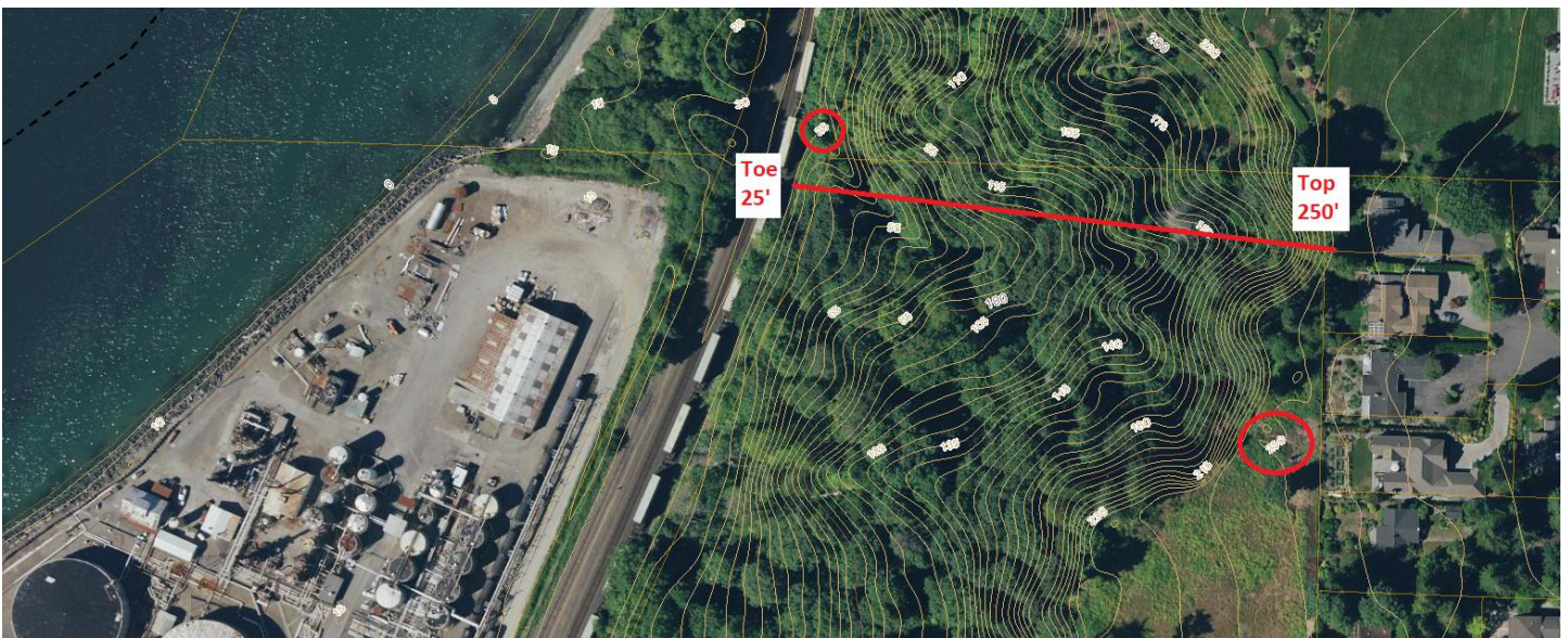
Figure 1 – Slope Height above North End of Point Wells Site (Snohomish County GIS)
