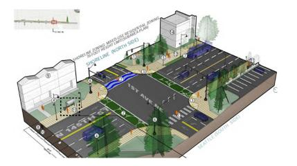
Recommendation is that a standard crosswalk pattern, rather than a decorative pavement marking, be used on all legs at the traffic signals
