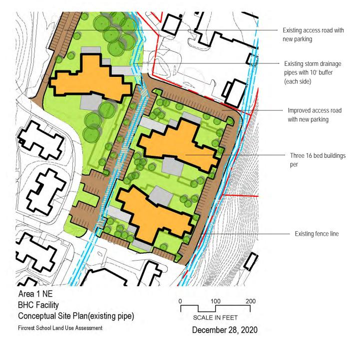
Figure 24 Diagrammatic site plan for a behavioral health center in the Northeast Corner (Area 1)
