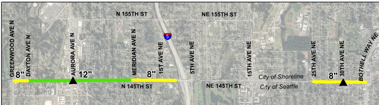
Figure 18 - New Mains and Connections, Alternative B3
