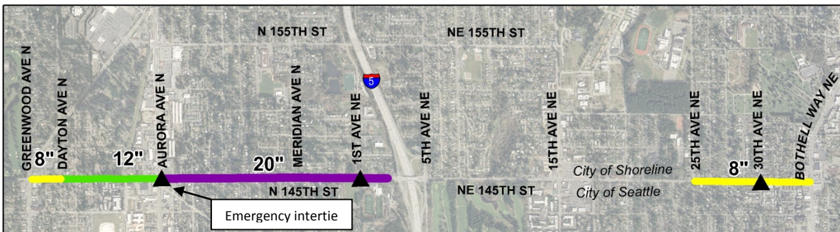
Figure 17 - New Mains and Connections, Alternative B2
