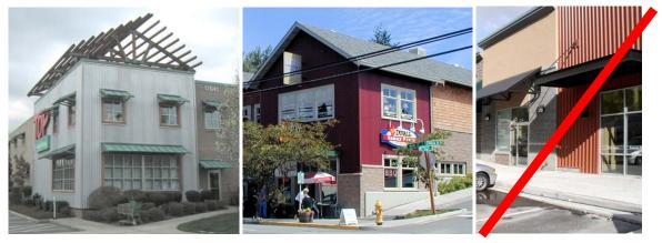
Figure 20.92.200(B). Proper (left and center images) and improper (right image) use of metal siding. The left and center images use masonry or concrete near the ground and proper trimming around windows and corners. The orange metal siding in the right image extends to the ground level.
