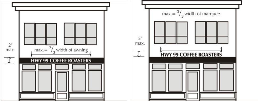
Figure 20.92.280(1). Examples of signs placed in front and on top of marquees.
