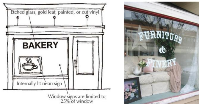
Figure 20.92.300. Window sign standards and an example.
