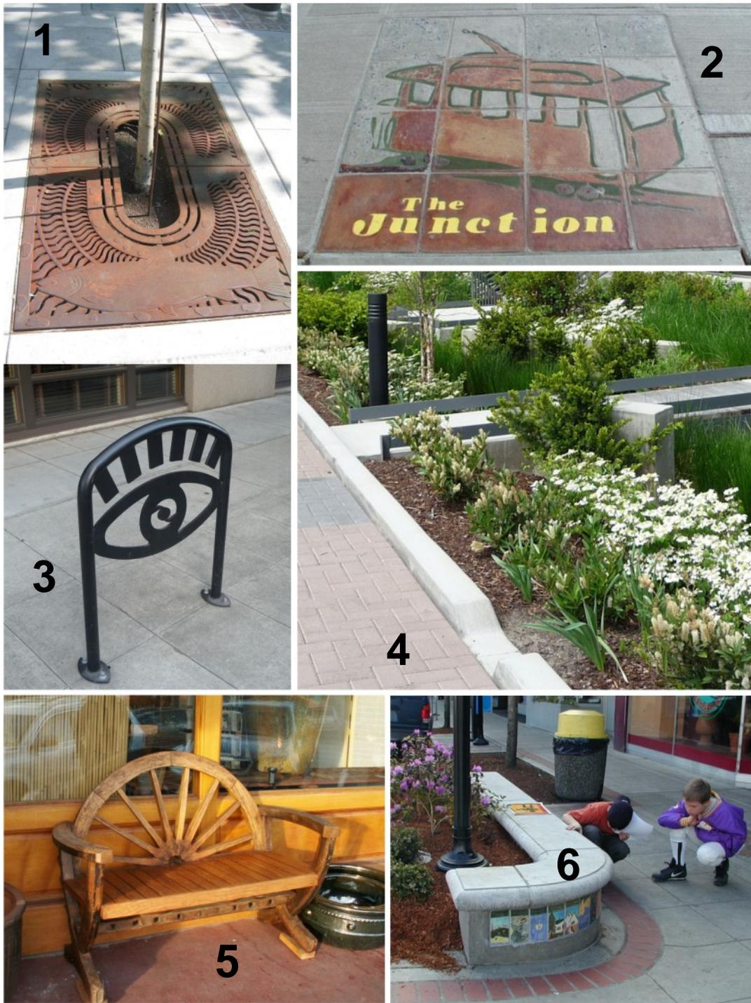
Figure 20.92.060(D)(2)(a). Desirable streetscape amenity examples. Image 1 includes a decorative tree grate; image 2 includes decorative artwork/paving related to the character and identity of the area; image 3 is a decorative bicycle rack; image 4 includes a rain garden planting strip; image 5 is a decorative bench; image 6 includes a sitting ledge incorporating student artwork.
