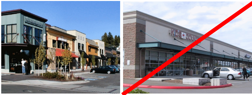
Figure 20.92.180(B). Good and bad storefront articulation examples.
