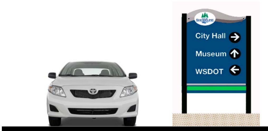
Fig 10. Wayfinding signs can be located in medians, behind sidewalks, or on poles
