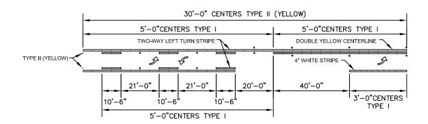
TYPICAL TYPE I AND TYPE II TRAFFIC BUTTON (4") INSTALLATION DETAILS
